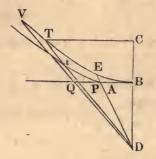
With center D and vertex B, describe the rectangular hyperbola B T V, cutting the lines D A, D P, D Q produced in E, T, V.
